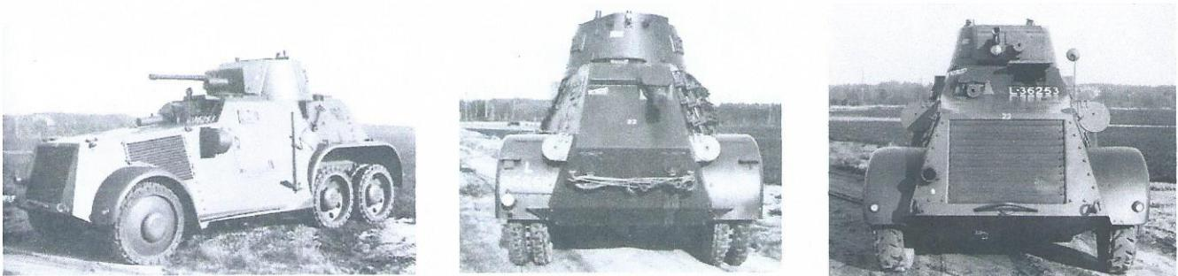
M-38 (Landsverk 182); marked with licence plates on the front and rear, red-white-blue plates with registration numbers on the front and rear, and two-digit vehicle numbers in white on all sides and on the turret sides. These markings were used in 1938-39. Overall color deep dark (olive) green.
